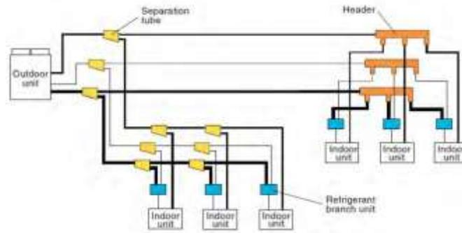
Figure 6: Typical Layout of a VRF System (taken from ASHRAE)
